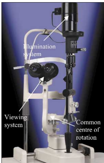
Figure 1 Basic slit lamp design (picture courtesy of Topcon)
